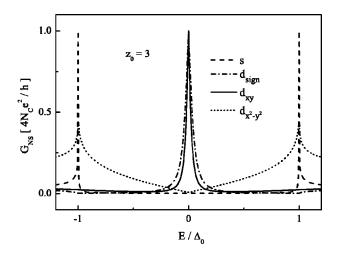
FIG. 3. The conductance is plotted as a function of *E*, where  $z_0 = 3$ . The anisotropy of the pair potential in  $d_{xy}$  symmetry is taken into account only through the phase factor  $e^{i(\phi_- - \phi_+)}$  and *k* dependence of the pair potential is neglected in the dash-dotted line. The  $d_{xy}$  symmetry is fully taken into account in the solid line. The conductance for  $d_{x^2-y^2}$  symmetry is amplified by five times in the dotted line.
